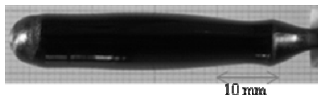
Figure 1: \text{CaFeO}_{3.8} single crystal grown in Ar atmosphere
